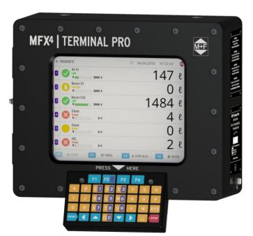
In order to ensure optimal ease of use, it is equipped with a configurable graphic, high-contrast and full-colour display. It also offers a user interface in several languages and displays all of the attached system's process data.
